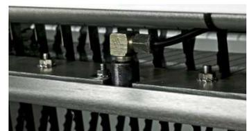
Optional automatic oil lubrication system prevent sticking of crumbs on blades. In particular recommended for slicing darker bread types.
