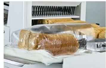
After slicing of the bread, a bag blowing device automatically opens the plastic bag. Sliced bread is inserted manually in one natural movement, saving considerable time.
