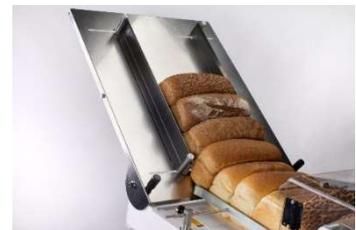
Optional chute for extra bread infeed storage for up to 15 breads. Chute with side guide strips for different sizes of bread and can be folded down completely when not in use.
