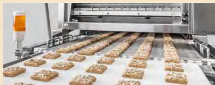
Seed depositors and round and long moulding units for bread and bread rolls
