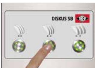
The customer selects the cutting thickness between "thin" (8 mm), "medium" (10 mm) and "thick" (12 mm) at the push of a button. Other thicknesses are available on request (max. 3). After pushing the button, the machine starts automatically.
