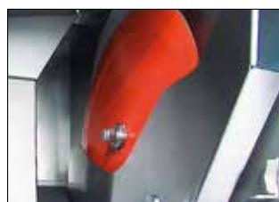
The blade guard offers safety during the cleaning. The blade guard is part of the standard equipment. It belongs automatically to the extent of delivery.
