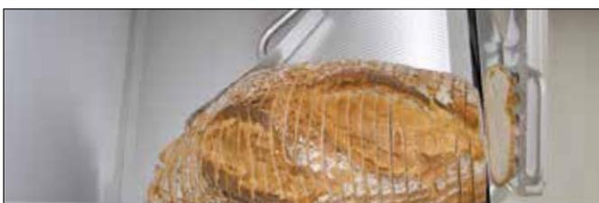
The automatic slice holder (TREIF patent) supports the slices during the slicing process, making it easier to remove the bread. It can be immediately placed into a bag. The slice holder swivels back automatically after the removal of the sliced bread.
