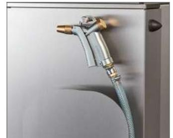
A hand spray allows easy cleaning of the tank, paddles and scrapers.
