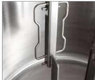
A performing mixing tool (unchanged form, patented) ensures an homogeneous mixing from top to bottom.
